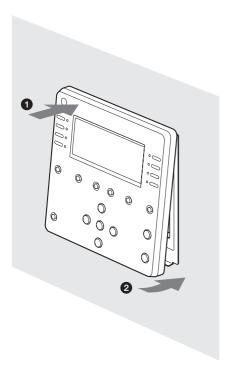
**4** Fix and tighten the Keypad mounting screws as shown below.
